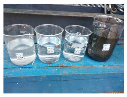
Left -Raw produced water: Center-Permeate- housing 1 and 2; Quality-1 ppm oil, <1ppm TSS,<1 micron: Right – Oil separated in Housing and automatically drained from housing
