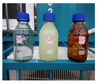
Right: Raw water with high amount of free oil Center: After Nitrogen Induced Gas Flotation to remove free oil. 2000 ppm emulsified oil RSL Membrane permeate: <25 ppm oil.
