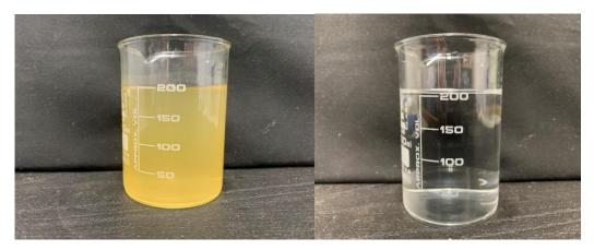
Produced Water treatment-Raw water 132 NTU Permeate <0.5 NTU- Permian Basin New Mexico
