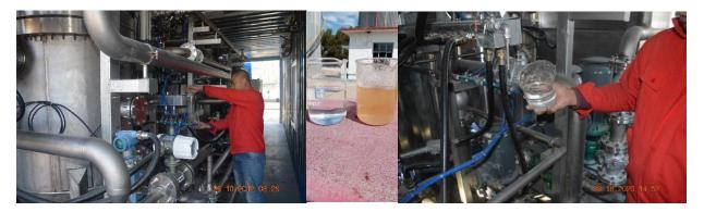
Left- Operator taking sample of raw water- Two Membrane Housings 12.5 m3/hr each Right- Operator taking sample of permeate from Membrane housing 1
